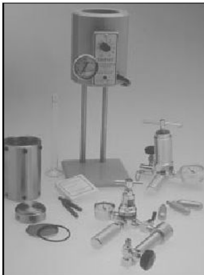
Figure 8: HTHP filter press (API #1 style) (disassembled).
