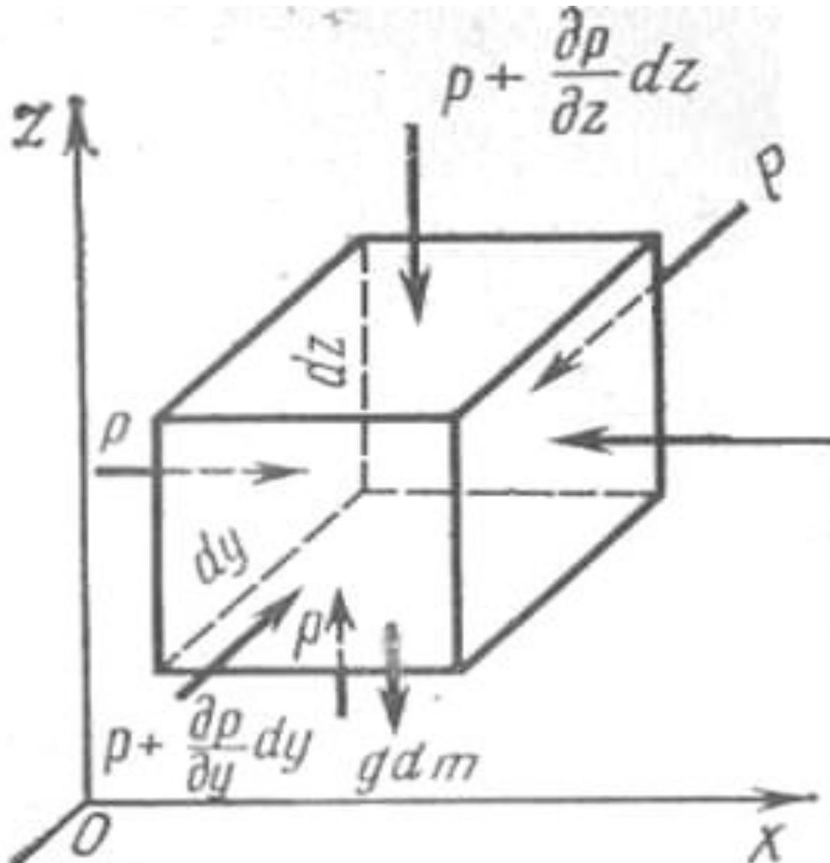
$$\begin{aligned} -\partial p / \partial x &= 0; \\ \partial p / \partial y &= 0; \\ -\rho g - \partial p / \partial z &= 0. \end{aligned}$$
