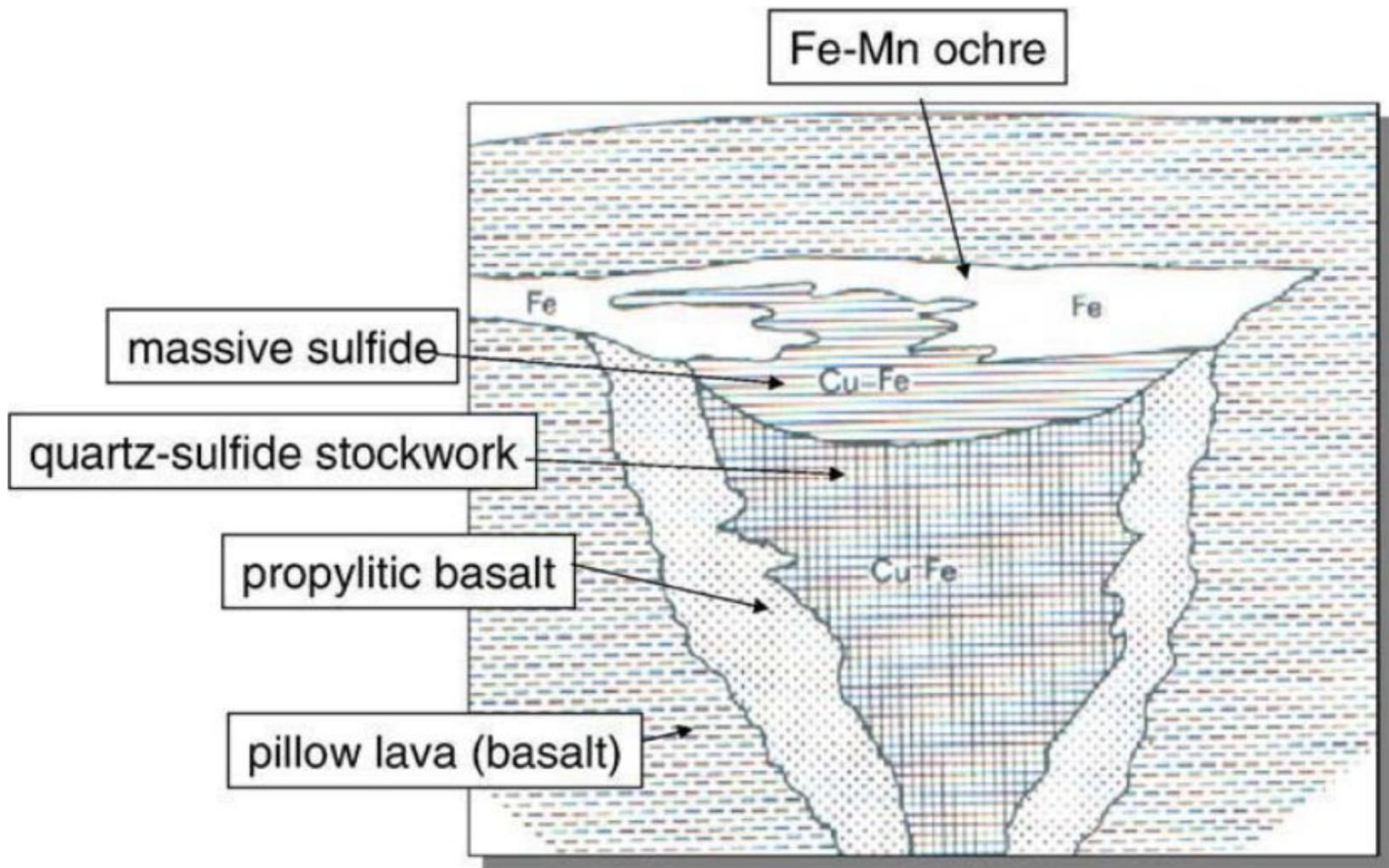
**Fig. 3.6. Position of Fe–Mn ore on top of the volcanic massive sulfide deposit of the Sha Mine Cyprus.**
