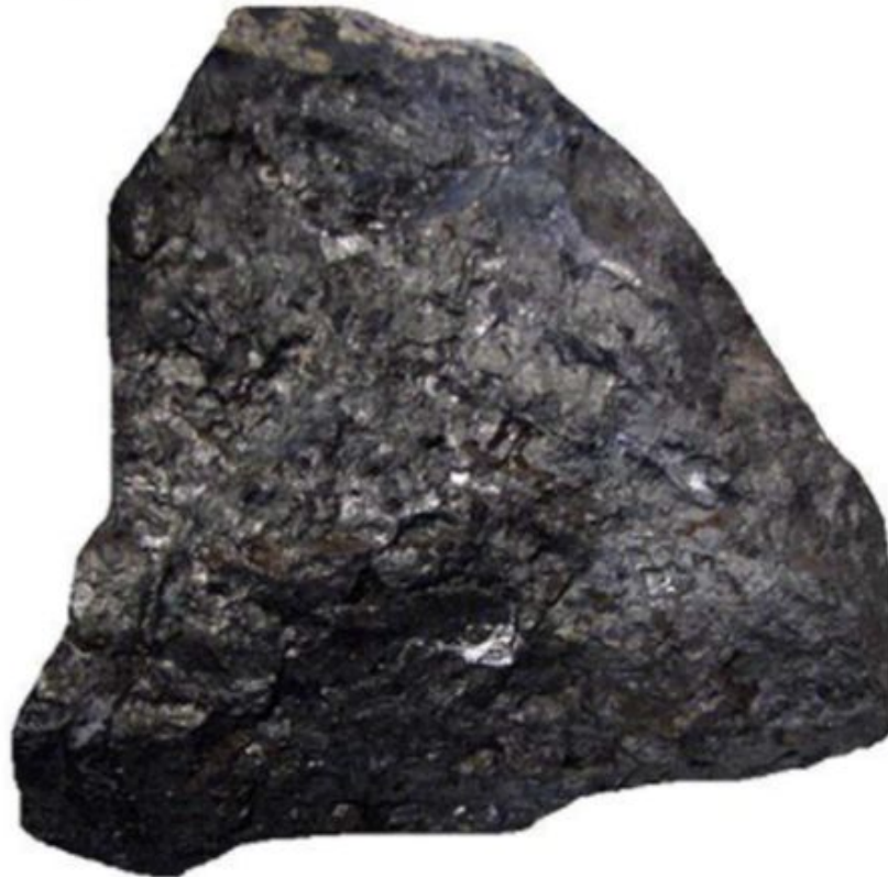
Fig. 3.3. The Kalahari manganese ore field (South Africa). a) Massive oxidic Mn ore b) Mn ore consisting of very fine-grained, banded braunite-kutnahorite lutite with laminae of Mn-calcite
