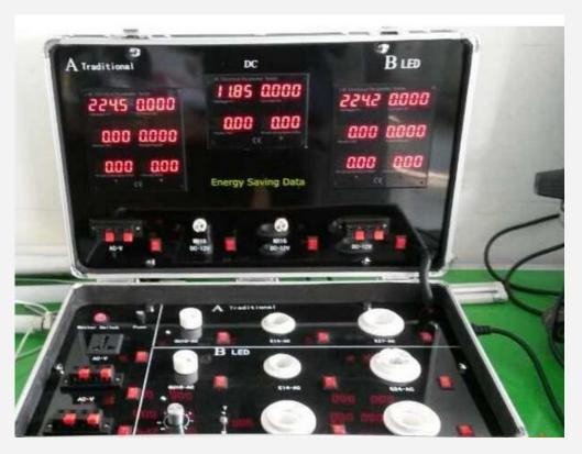
This instrument can check the power factory, wattagge, vottage.
