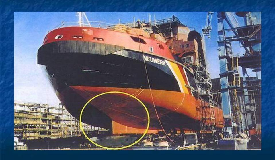
The depth of ship's bottom or keel below the waterline is draught. The beam of the ship is the distance between the two sides.
