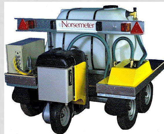
Norsemeter Roar friction measurement trailer
