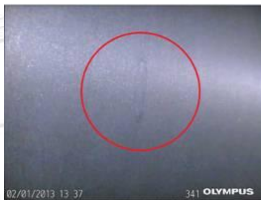
This is the impressed burr under a normal white light inspection
