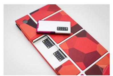
Project Ara is the codename for an initiative that aims to develop an open hardware platform for creating highly modular smartphones.  It would allow users to swap out malfunctioning modules or upgrade individual modules as innovations emerge, providing longer lifetime cycles for the handset, and potentially reducing electronic waste
