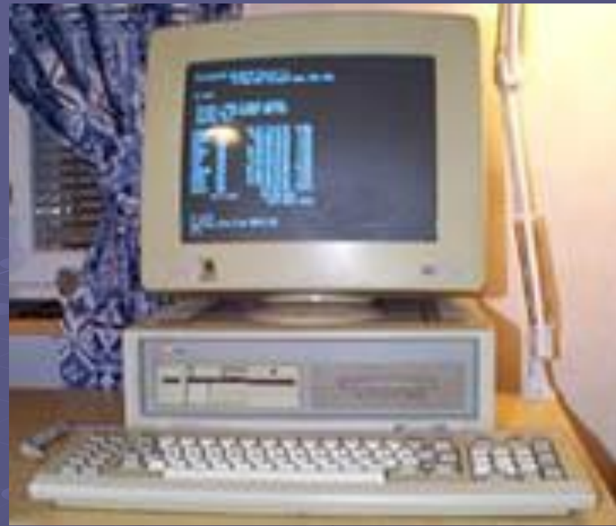
Amstrad 8086 (PC) 512K Memory, 32 MB HD, CGA-monitor and graphics card, One 5 1/4" drive, One 3,5" drive (720Kb disc's)
