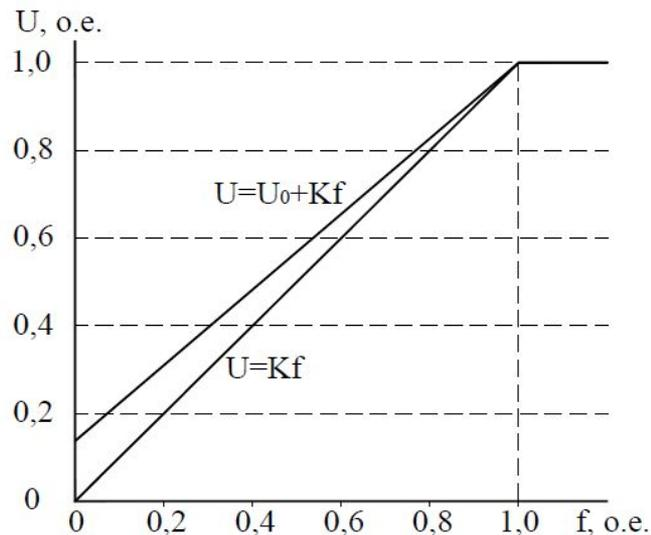
$$\left. \begin{aligned} U &= Kf, \\ U &= Kf^2, \\ U &= U_0 + Kf, \end{aligned} \right\}$$
