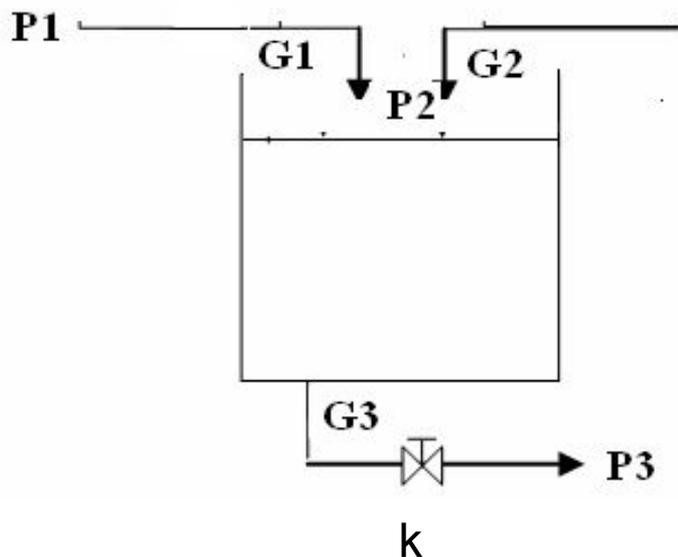
$$(1) \quad \begin{aligned} G1 + G2 &= G3 \\ G3 &= k \cdot \sqrt{\gamma H + P2 - P3} \end{aligned}$$
