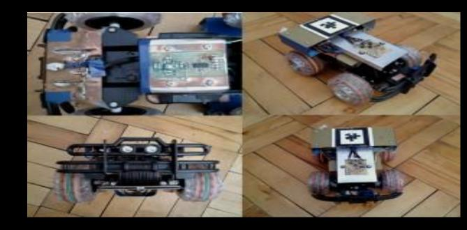
Teams develop their own algorithm of the device choose the components and design interaction of these subsystems provide printed circuit board mounting of components involved and the creation of a special software for device management.
