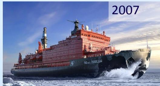
The OK-900A reactor plant with two **171 MW** reactors is installed in nuclear ice-breakers “Arktika”, “Sibir”, “Rossiya”, “Sovetskiy Soyuz”, “Yamal” and “50 Let Pobedy” with the MPP power of **75 000 hp**.
