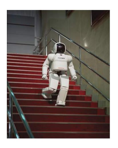
ASIMO is a humanoid robot cre ated by Honda MotorCompany . Standing at 130 centimeters and weighing 54 kilograms. Th e robotresembles a small astro naut wearing a backpack and c an walk or run on two feet at s peeds up to 6 km/h. Officially, the name is an acron ym for "Advanced Step in Inno vative **MO**bility". Honda's offici al statements. TonyMcNicol. Th ese bots were made for walkin g: Honda's bold new bots are h eaded into your home.
