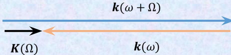
$$\Delta k = k(\omega + \Omega) - k(\omega) - K(\Omega) = 0$$
