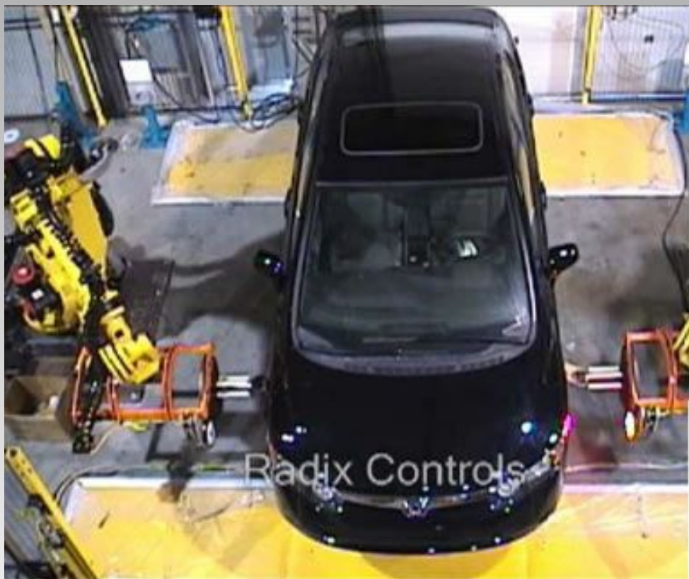
Vision-guided robots position nut runners on wheels
