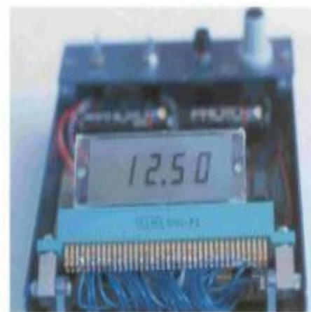
The first twisted nematic display (TN/LCD) prototype, made in 1971.
